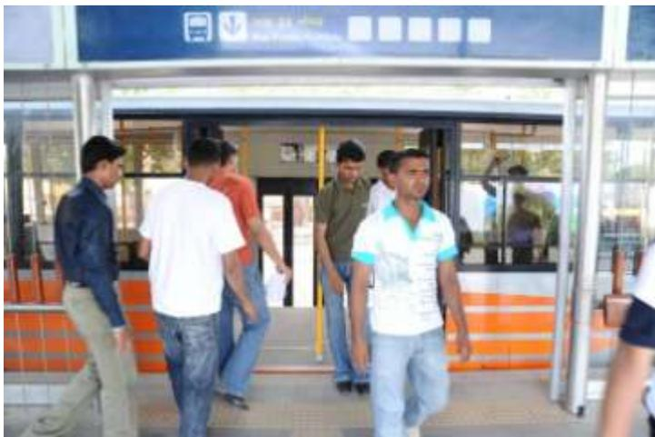
*Picture showing Wide Automatic Doors on the Buses and Stations matched to enable level boarding*
